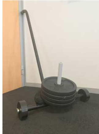
Figure 4: A rudimentary test cart used to generate indoor rolling noise.
